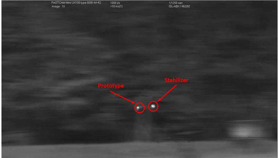
Figure 73: Video Recording 10 ms from the Firing Instant for the 2205 MHz Prototype.
